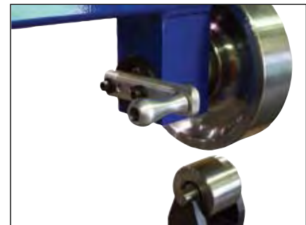
Roller Cam Action Release Lever on Top Wheel
