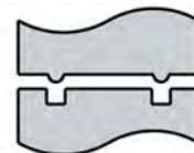
TP1008-1PS 1/8" Pin Stripe (7/8" center to center bead)
