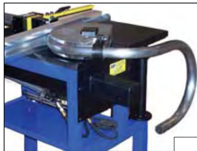
Compound bends are easier with redesigned top.
