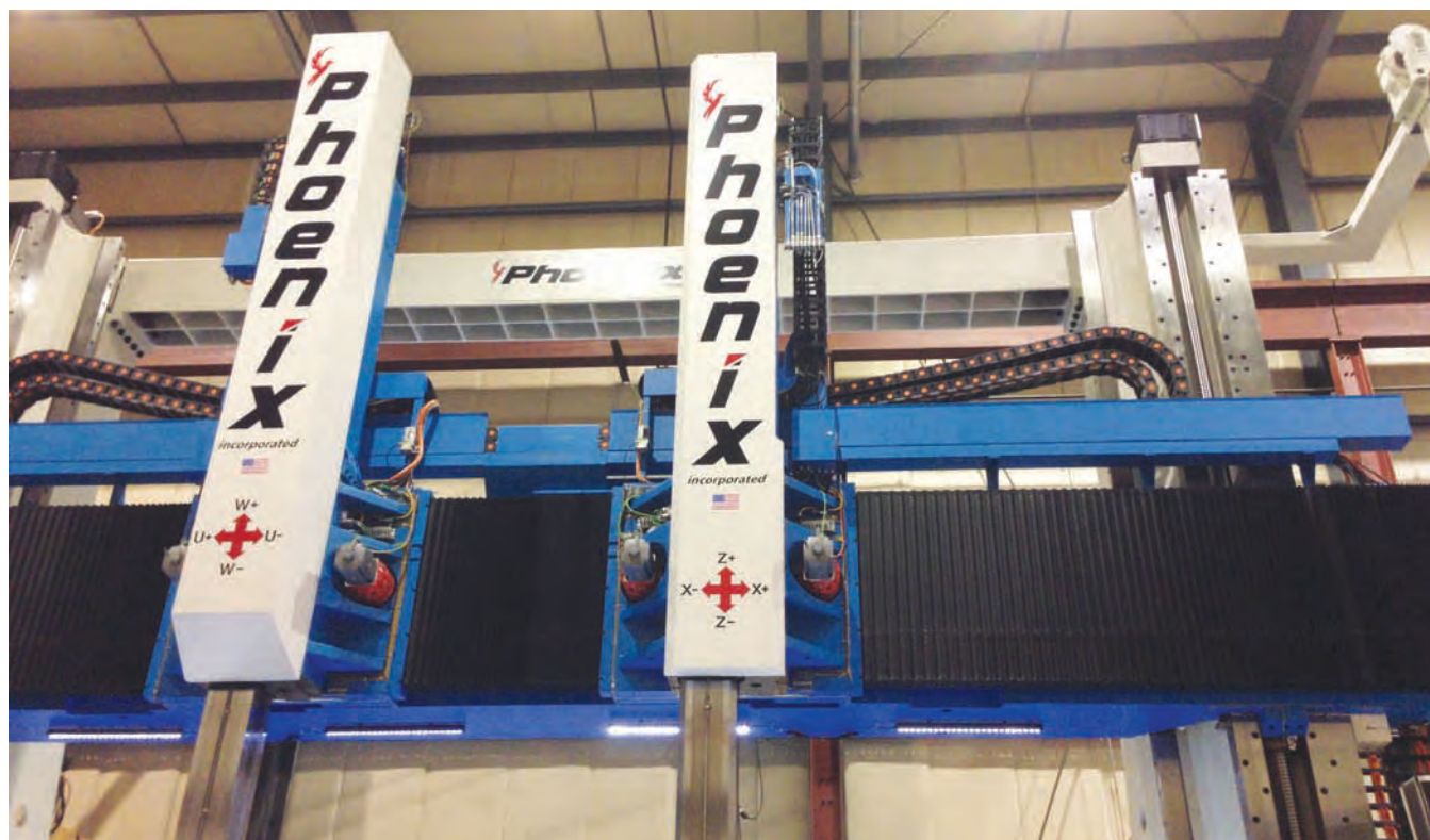
Bellows type way covers and plastic cable carriers with long travels on large vertical machining center.
