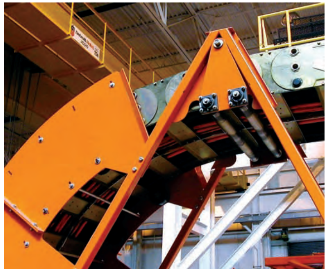
Blow-molding application with Gortrac steel XL carrier with patented "Walker" support system to reduce shock load by preventing link lock-out.
