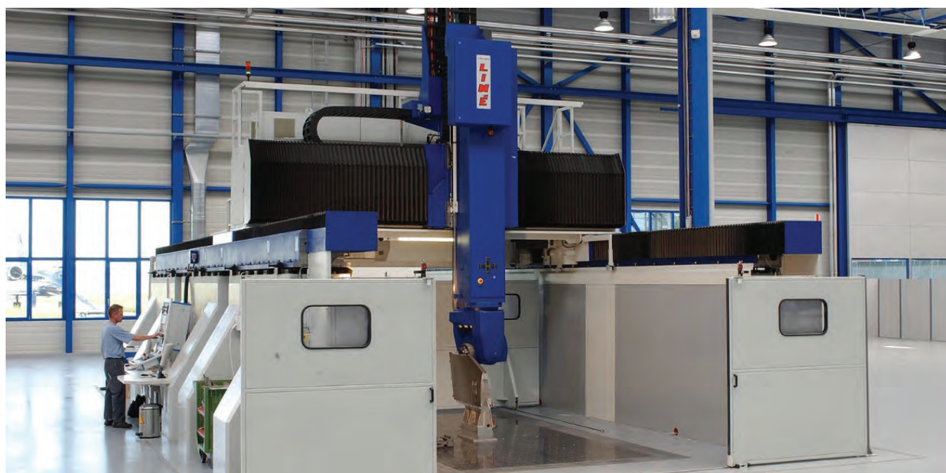
Bellows type way covers on large machining center.
