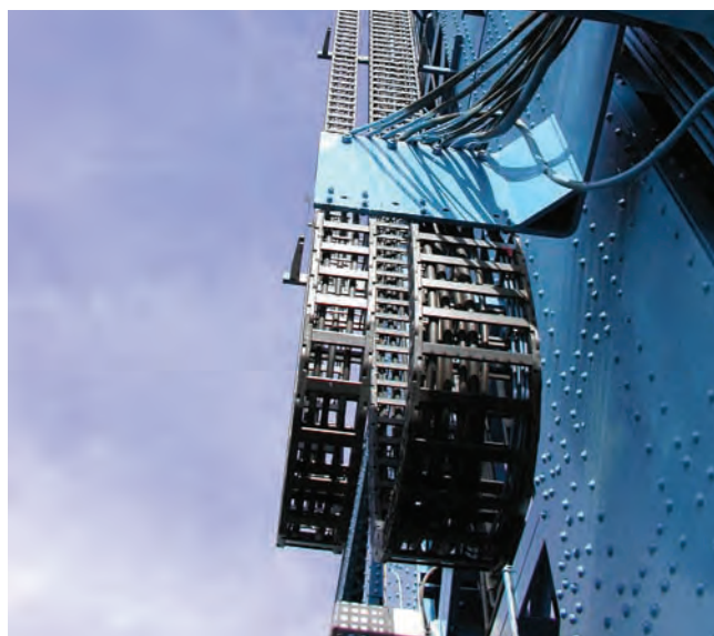
Nylatrac Modular TL carriers, with anodized aluminum crossbars for added strength in heavy wind conditions, maintain the lines for electric and hydraulic controls on a vertical lift bridge. Shown: The Main Street Bridge in Jacksonville, Florida.
