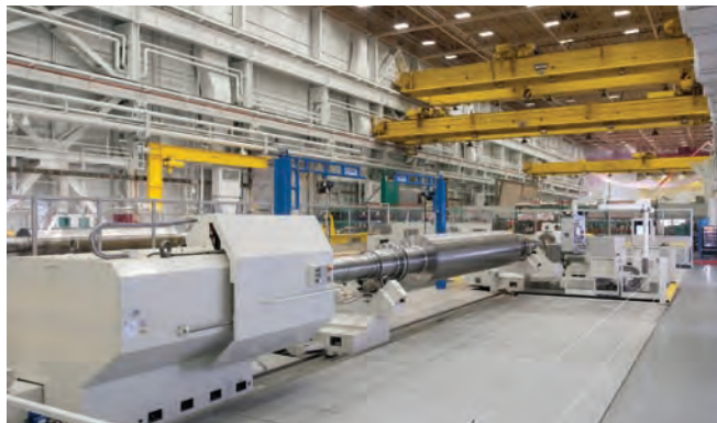
Steelflex® walk-on duty covers have been used for decades for personnel safety and machine protection, in the covering of machine ways and inspection pits.
