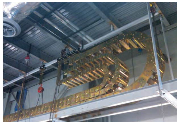
Nested steel carrier assembly supplied complete with long travel guide trays and trolley system, and custom steel crossbars.
