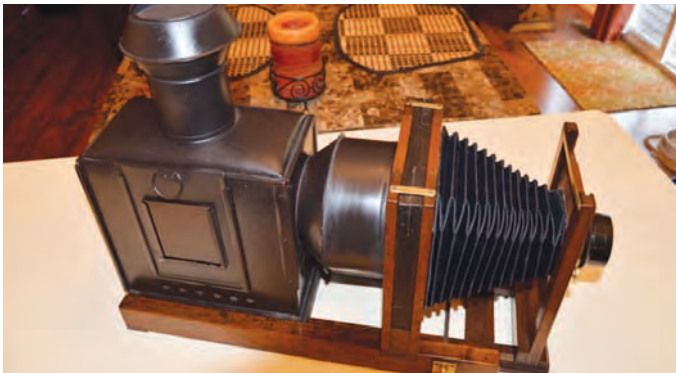
Light-tight bellows used on a photo enlarger, folded construction.
