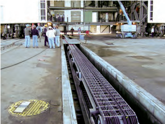
Custom stainless steel Gortrac® LRC carrier system with rolling carriage for a rocket launch system in California. Driven end modified for customer's application requirements.
