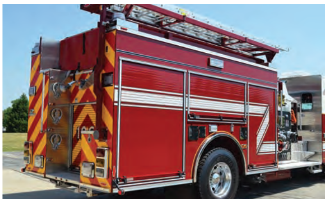
Gortite® aluminum roll-up doors are used on fire and emergency vehicles, work/utility trucks, and other commercial vehicles.
