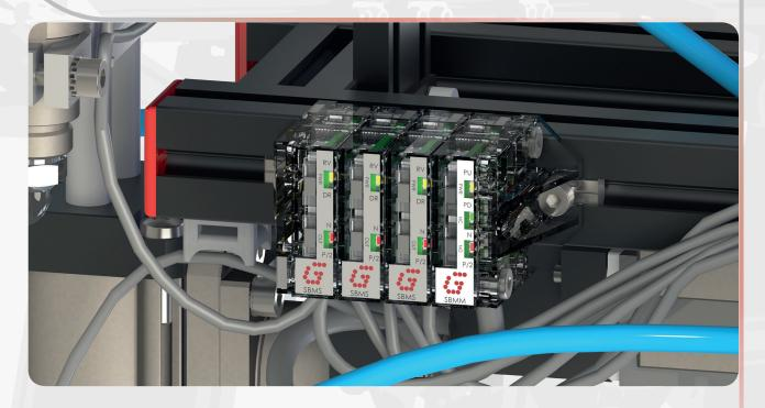
An innovative way to consider the EOAT sensor boxes. The modular sensor box SBM will allow to connect in series from 2 to 20 switches in any configuration (PNP/NPN, NA/NC), getting a single signal to allow EOAT operations.
