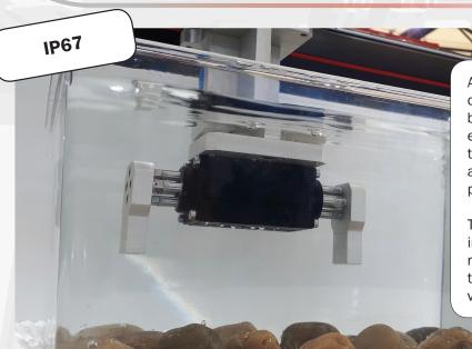
A parallel gripper, specifically designed to provide the better performances in harsh environments, internally sealed to preserve from dust, oil and also one meter underwater with protection class IP67.
