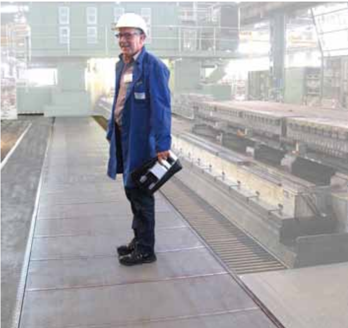
Steelflex walk-on duty covers have been used for decades for personnel safety and machine protection in the covering of machine ways and inspection pits.
