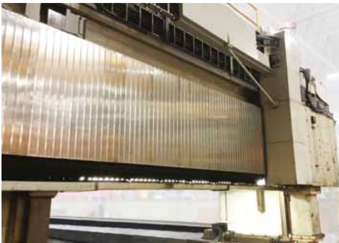
Bellows with stainless steel blades for machine way protection have been successfully applied in vertical, horizontal and crossrail configurations.
