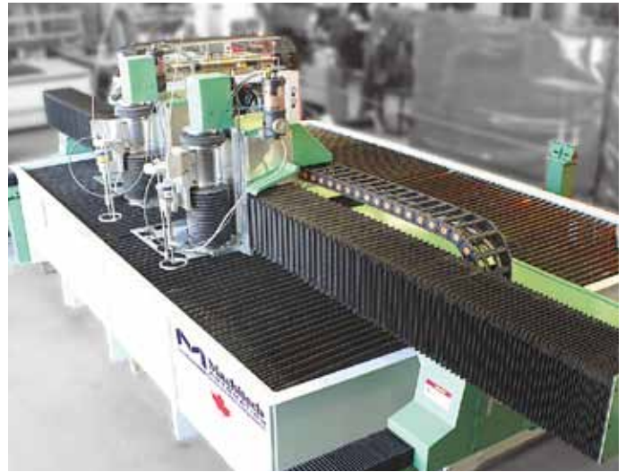
Bellows and Nylatrac cable carriers on a waterjet machine.
