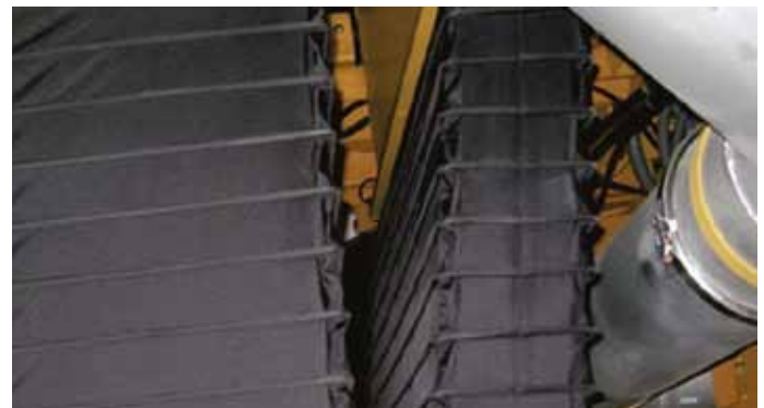
Gorframe bellows for flexible air ducting on a heavy truck.
