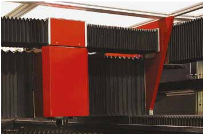
Special laser beam bellows are used in horizontal and vertical configurations.
