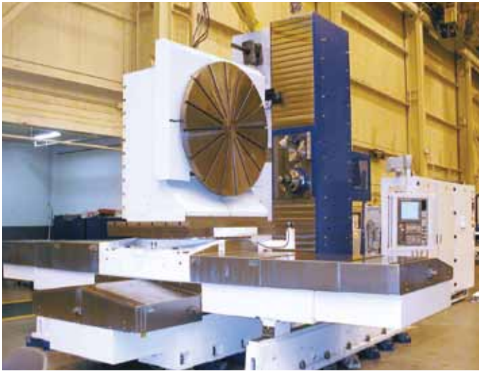
Telaflex steel covers and bellows with blades are used here to protect the machine ways of a horizontal boring machine from accumulating chips and liquids.
