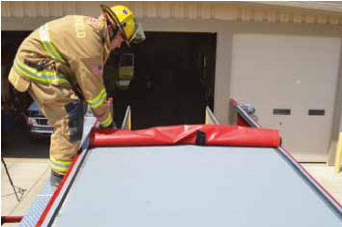
Heavy-duty roll-ups can be applied to fire truck hose beds as a retractable cover and also as a walk-on surface when not in use.
