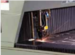
Light-tight bellows for laser beam path
