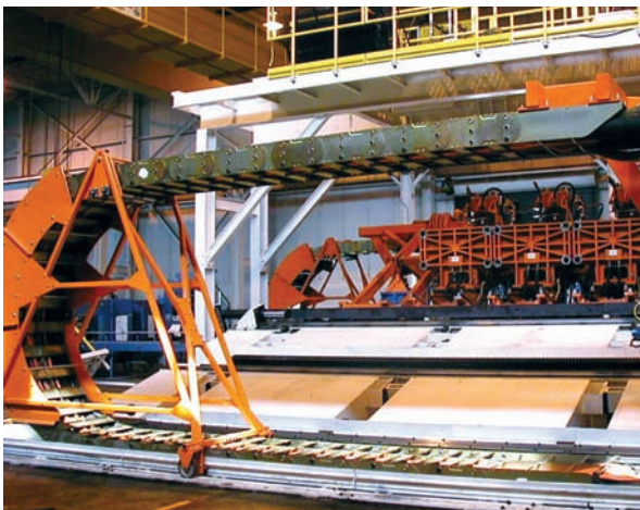
Blow-molding application with steel XL carrier with patented "Walker" support system to reduce shock load by preventing link lock-out.
