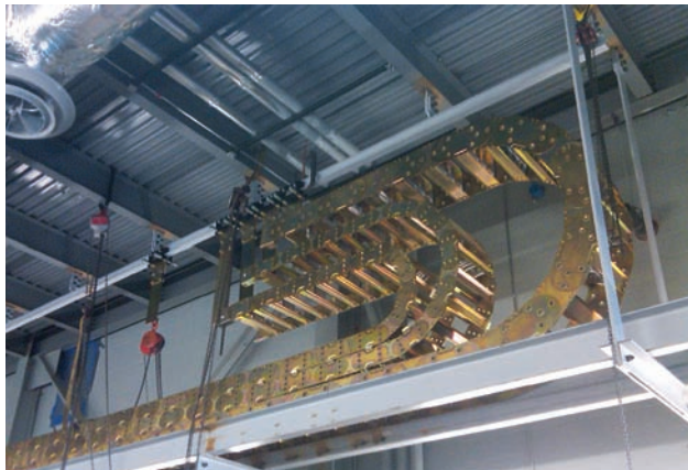
Nested steel carrier assembly supplied complete with long travel guide trays and trolley system, and custom steel crossbars.
