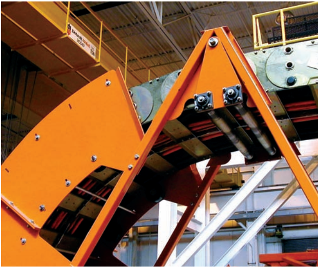
Blow-molding application with Gortrac steel XL carrier with patented "Walker" support system to reduce shock load by preventing link lock-out.
